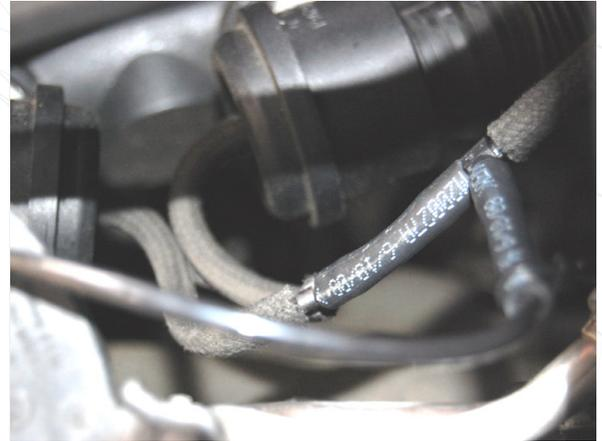
**17** Check that all lines are secure, pull excess slack back into the cabin, and replace the cover back over the brake fluid and firewall area. We are now done under the hood, your tubing should look like this now.
