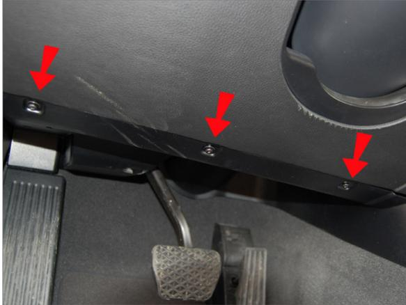
**12** Go back out to the car, and remove the lower dash cover below the steering wheel by removing the three #20 torx screws shown above. Then lay this cover into the footwell.
