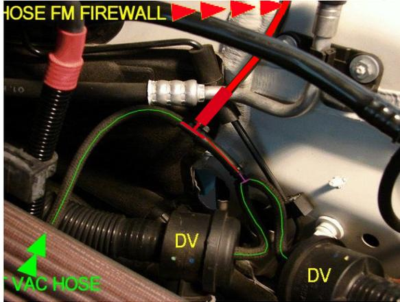
**16** Find the "Y" connector that splits the vacuum hose directly before the diverter valves. Unplug the bottom side of the "Y" and insert the supplied vacuum T and tubing as shown. Shove at least a quarter inch of the nylon tubing into this new tap, and secure with a zip tie.
