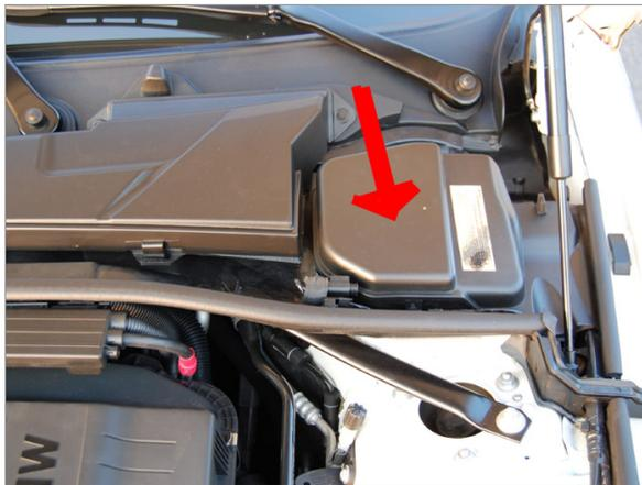
**14** Pop the hood, and remove the driver side cover which hides the brake fluid resevoir. This cover just has clips on either side, and a rubber tab that hold it in place. After removing this cover, set it aside, this is all you need to remove in the engine bay area.
